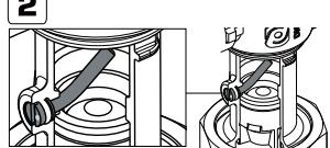
After a complete filling and venting, turn the screw on the check valve back to its normal operating position, picture 2 and set the circulation pump operation to recommended position.
