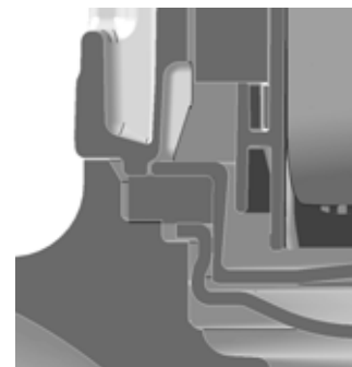
Fig. 37 Sectional drawing showing sealing principle of gasket
